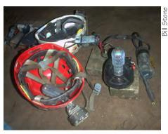
In-cave recharging of electrical gadgets. We used Mil-surplus lithium-SO4 primary batteries (the dark green blocks) to recharge helmet STEN lights, primary dive lights (black cylinder to the right, from NiteRider), Mk6 rebreather batteries (clear plastic cylinder), as well as Underwater Kinetics eQ-LED underwater lights. These two blocks provided all electrical power for the 7-1/2 days spent working from Camp 4 on the final push in 2009.
